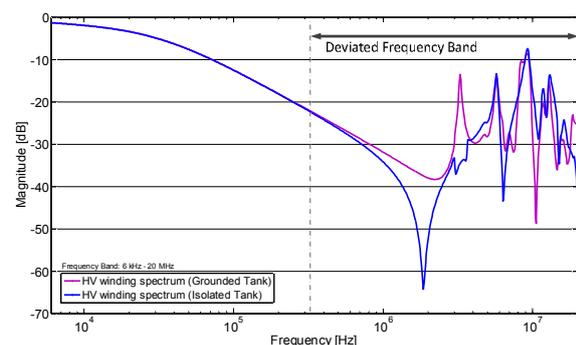
Fig. 5. FRA spectra of HV winding for isolated and grounded tank.
