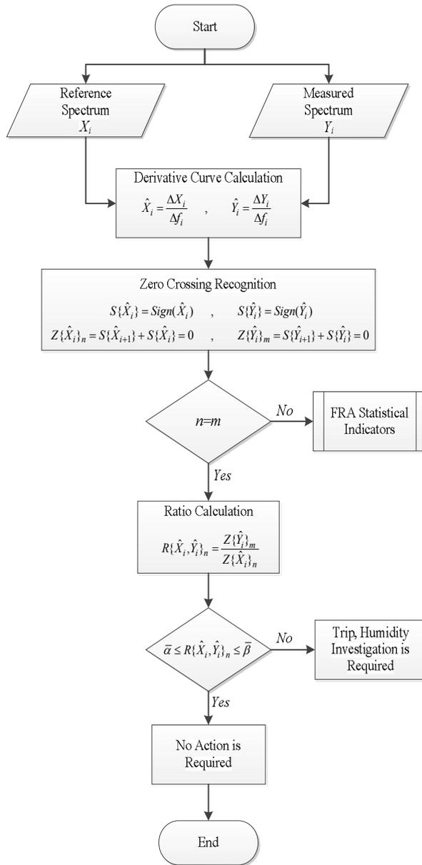
Fig. 6. The chart on preliminary calculation on FRA traces to distinguish insulation deviation from winding deformation;  $X_i$  and  $Y_i$  are defined  $i^{\text{th}}$  samples in FRA fingerprint and measured traces.
