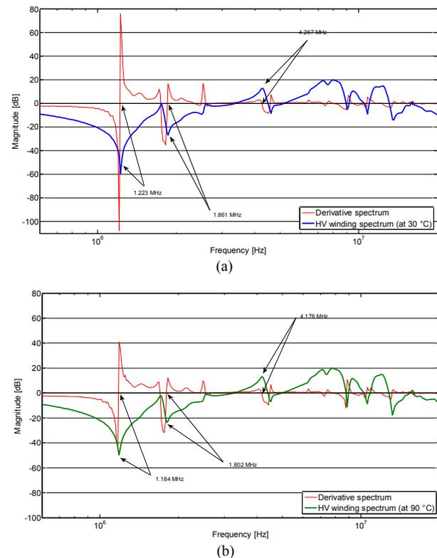
Fig. 7. Reference and derivative spectra for HV winding of glassy model transformer, (a) Spectra at 30°C, (b) Spectra at 90°C.
