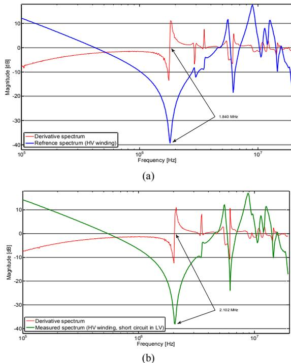
Fig. 8. HV winding spectra (a) Reference spectrum and its derivative (100 kHz – 20 MHz), (b) Measured spectrum and its derivative (100 kHz – 20 MHz).
