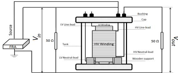
Fig. 2. Implemented FRA measurement setup on glassy model transformer.
