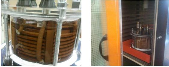
Fig. 1. Manufactured glassy air-core transformer.
