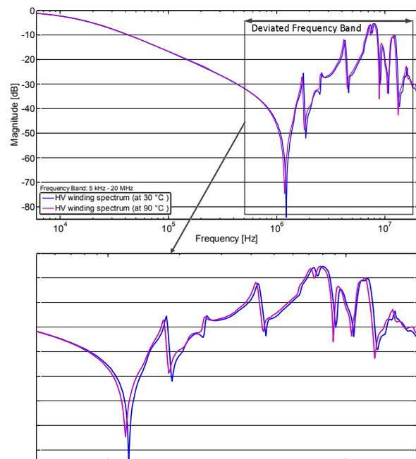
Fig. 3. FRA spectra for HV winding due to moisture migration from paper into the oil insulation at 30°C and 90°C.
