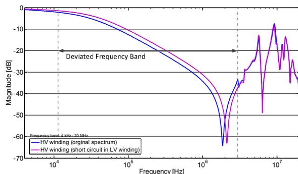
Fig. 4. HV winding frequency response spectrum when LV winding is open-circuited (original spectrum) and short-circuited..
