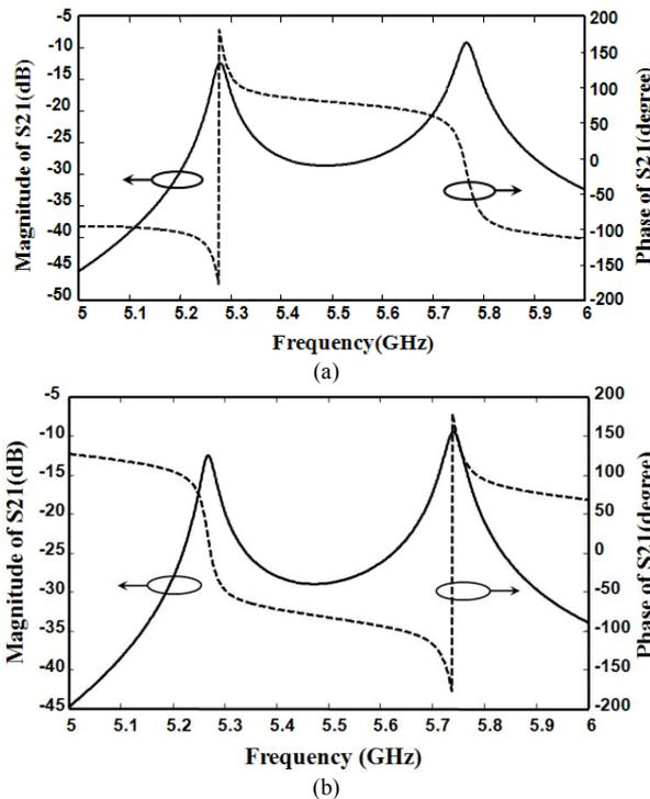
Fig. 4. Phase and magnitude response of internal coupled SIW resonators. (a) positive coupling (b) negative coupling.
