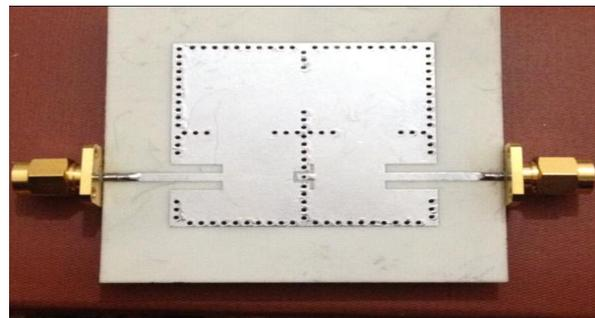
Fig. 8. Prototype of the fabricated SIW filter.
