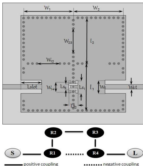
Fig. 1. Structure and coupling scheme of SIW cross coupled BPF.
