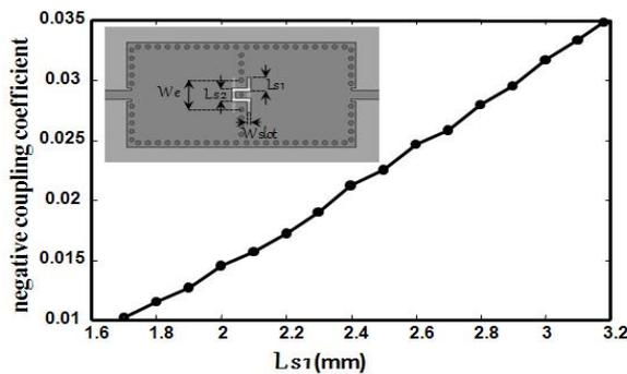
Fig. 6. Negative coupling coefficient between two proposed SIW resonators ( $d=0.45$ mm,  $p=1.7$ mm,  $W_c=3.2$ mm,  $W_{slot}=0.5$ mm,  $L_{s2}=2.4$ mm).
