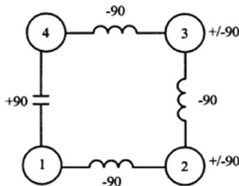
Fig. 3. Two paths for travelling signal from source to load.
