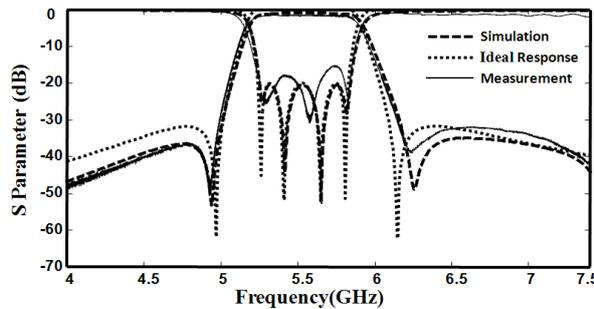
Fig. 9. Measured, simulated and ideal responses of proposed SIW quasi-elliptic BPF.
