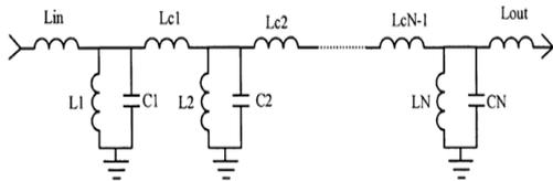
Fig. 2. Equivalent circuit of filter.
