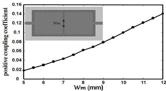
Fig. 5. Positive coupling coefficient between two proposed SIW resonators ( $d=0.45$ mm,  $p=1.7$ mm).
