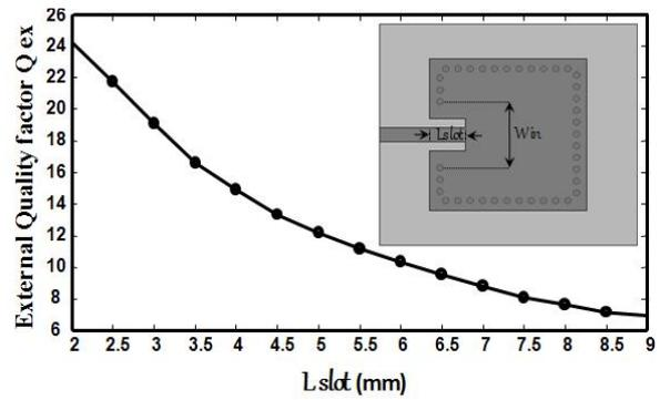
Fig. 7. External Q-factor of the proposed SIW resonators ( $d=0.45$ mm,  $p=1.7$ mm,  $W_{in}=1$ mm).
